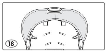
• Hook the elastic loops on each side of the pad onto the tabs in the seat back.
